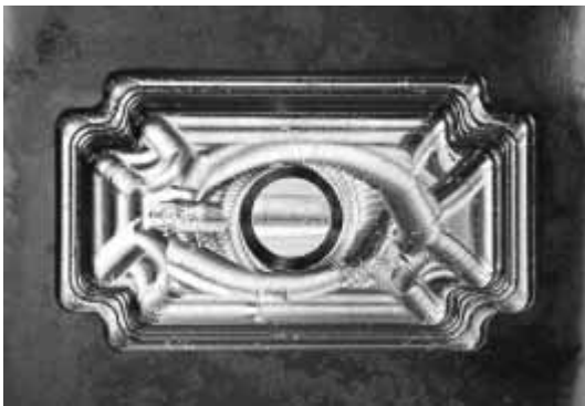
Fig. 10 Machined workpiece after rough and intermediate-rough cutting
