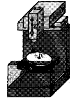
Fig. 1 Five-axis machine tool with a tilting rotary table
