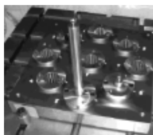
Fig. 2 The outlook of the jig plate and ball holders
