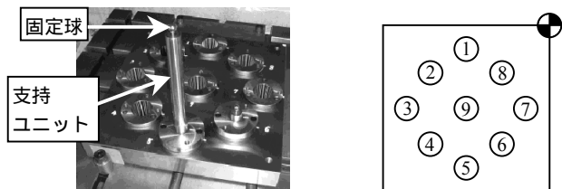
Fig.3 A jig for DBB measurements.
