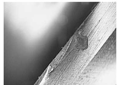
Figure 11. Comparison of tool wear observed by a CCD camera when the machining is finished
