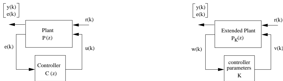
(a) Closed-loop system configuration of the problem (3.53) (b) Extraction of controller parameters K
